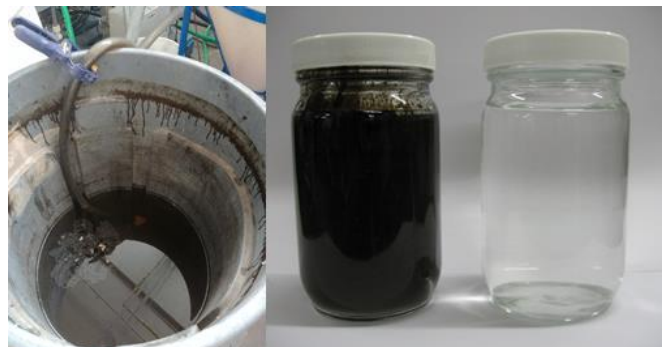
Bilgewater vs. Treated Effluent
