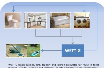
WETT-G treats bathing, sink, laundry and kitchen greywater for reuse in toilet flushing, laundry, cleaning and irrigation (or safe discharge to the environment). Contingency operations may elect to reuse treated greywater for showering.
