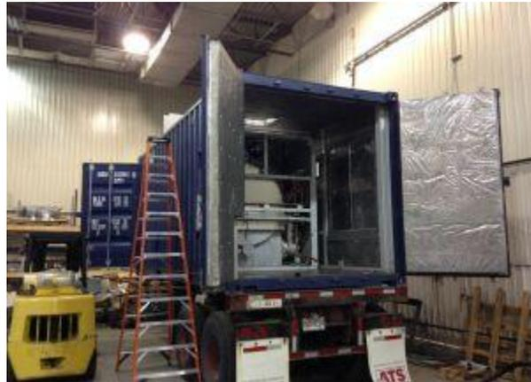
The STEP system being installed in a container ready for the shipboard trials
